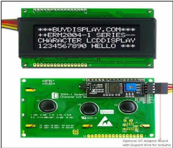
Gambar 4 LCD 20x4 I2C
