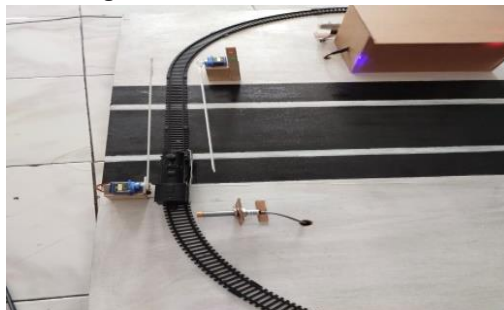
Gambar 16. Sensor Proximity 2 Mendeteksi Kereta Api
