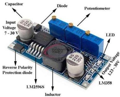
Gambar 6. Regulator converter
