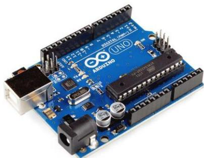
Gambar 1. Board Arduino Uno
